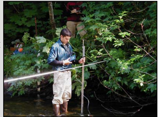
Jared using a Price AA flow meter (Gurly Meter) to measure stream velocity at USGS monitoring site.
